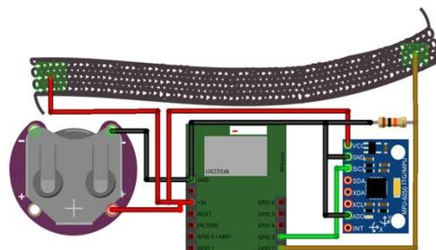
Figure 2: Fritzing diagram of chest strap.
